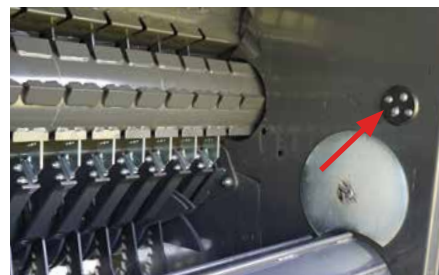
Moisture sensor located inside the bale chamber.
