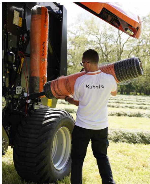
The smart net roll storage allows a comfortable horizontal loading.
