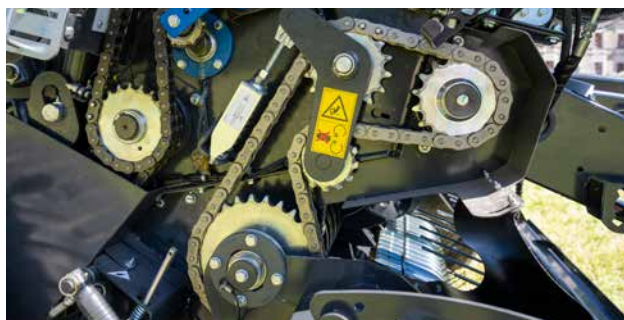
Rotor chain transmission with 1¼" pitch chains.
