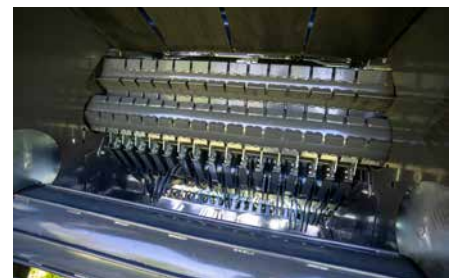
Profiled rollers provide instant bale formation and are equipped with self cleaning scrapers designed for working in all crop conditions.
