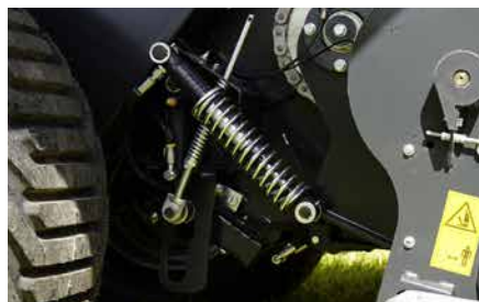
Hydraulic pick-up lift with integrated suspension system for accurate ground following.
